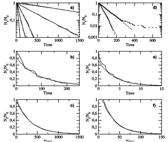
FIG. 5. Fraction of remaining orbits  $N_t/N_0$  in a function of the time  $t$  for the three-disk configuration (a)–(c) and the Hénon-Heiles system (d)–(f). For the three-disk configuration: (a)  $w = 1, 0.05, 0.02, 0.005, 0.001$  (from left to right). (b)  $w = 0.02$ ; (c)  $w = 0.005$ . For the Hénon-Heiles system: (d)  $E = 0.215$  (without KAM torus, in the hyperbolic regime),  $E = 0.19$  (with KAM torus, in the nonhyperbolic regime). (e)  $E = 0.4$ ; (f)  $E = 0.215$ .
