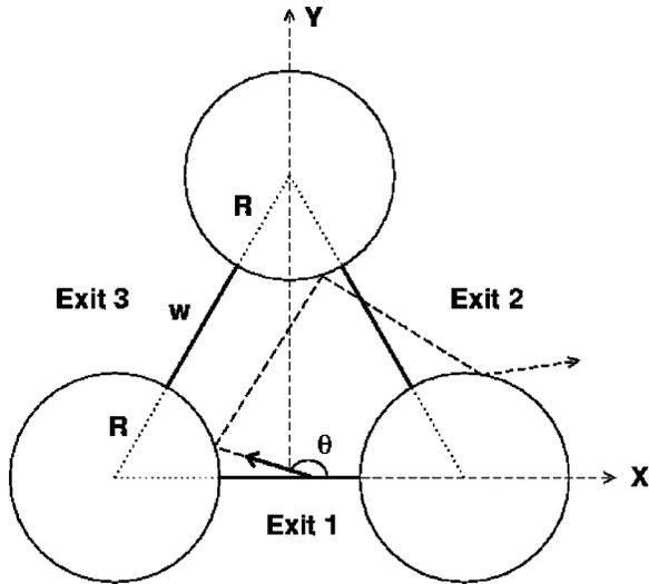
FIG. 1. Diagram of the three hard disk configuration. The only parameter that influences the system is  $w/R$ , where  $w$  represents the exit size and  $R$  the radius of the disks.
