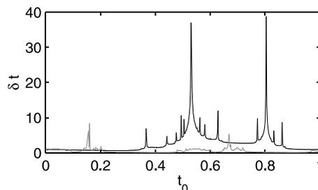
Fig. 4. Delay plots for the initial condition  $(x_0 = -5.0, y_0 = 0.01)$  at different starting times for the case of the static cylinder (curve in black) and for the case of the oscillating cylinder with amplitude equal to 0.2 length units and frequency the same as the one of the vortices (curve in gray).
