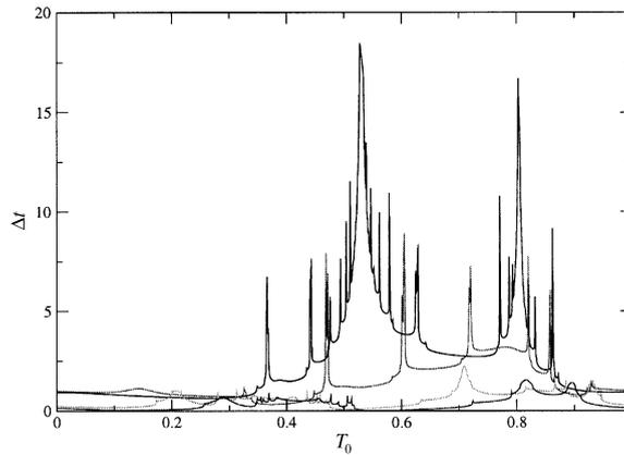
Fig. 2. Delay plots for the initial condition  $(x_0 = -5.0, y_0 = 0.01)$  at different starting times,  $t_0$ , as the rotational parameter is increased (the different values of  $\omega$  are 0.00, 0.10, 0.25 and 0.30). Note that as  $\omega$  is increased the height of the peaks are lowered. This shows that the trapping time of the trajectories decreases as  $\omega$  increases and hence their chaoticity diminishes.
