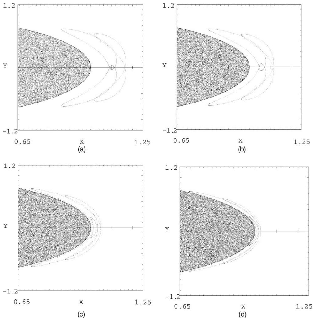
Fig. 1. The shape of the one-periodic orbits in the wake of the cylinder as the rotational parameter is increased. The different values of  $\omega$  are (a) upper-left panel, 0.00, (b) upper-right panel, 0.10, (c) lower-left panel, 0.25 and (d) lower-right panel, 0.30.
