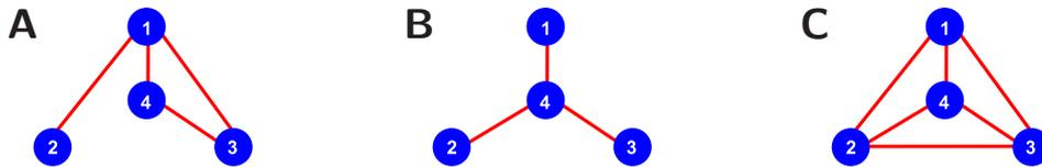
**Figure 1.8.** The clustering coefficient. The local clustering  $C_i$  and the clustering coefficient  $\bar{C}$  are here calculated for three simple examples. (A)  $C_{i=1\dots4} = \{1/3, \text{NA}, 1, 1\}$  and  $\bar{C} = 7/9$ . (B)  $C_{i=1\dots4} = \{\text{NA}, \text{NA}, \text{NA}, 0\}$  and  $\bar{C} = 0$ . (C)  $C_{i=1\dots4} = \{1, 1, 1, 1\}$  and  $\bar{C} = 1$ .
