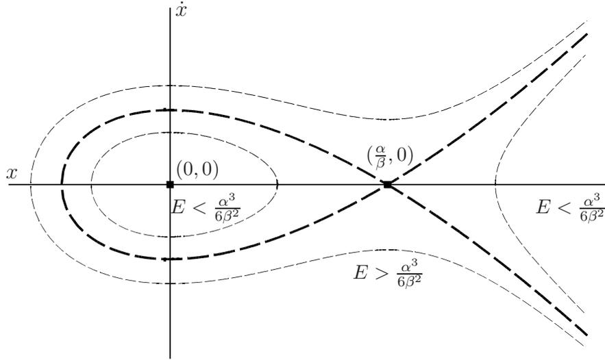
**Figure 4.2.** Phase space of the Helmholtz oscillator. The separatrix, in thick dashed line, is the stable manifold of an unstable periodic orbit. Therefore, bounded orbits correspond to the close curves around  $(0, 0)$ , that is, the orbits inside the separatrix, and the unbounded orbits are the curves outside.
