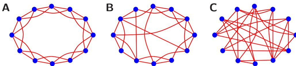
**Figure 1.14.** The Watts–Strogatz model. Here we show how a ring with 12 nodes and 24 links can be continuously transformed into a random graph by “rewiring” the ends of each link with probability  $p$ . The initial regular lattice (A) becomes a small-world network for halfway probabilities (B), and finally transforms into a random graph (C).
