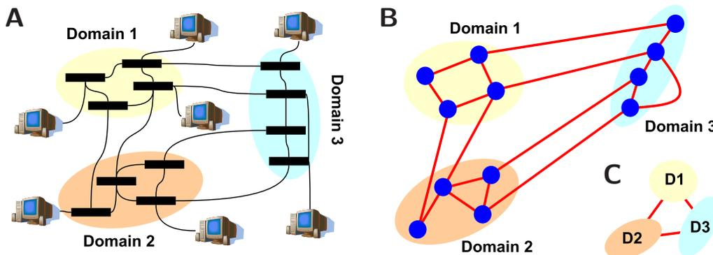
**Figure 1.1.** Schematic representation of the physical connections on the Internet. To transfer a file between two users, the packets encoding the file travel from the source host to the destination host via routers. (A) This figure depicts how hosts connect to routers (black boxes) and routers among them. (B) The corresponding network at the level of routers is drawn and, (C) the network at the level of domains.
