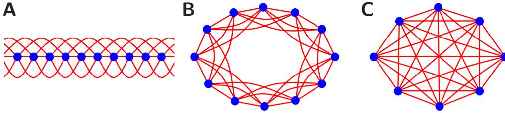
**Figure 1.11.** Lattices. (A) A one-dimensional lattice with each node linked to its 6 nearest neighbors (three on the left and three on the right). (B) The same lattice with periodic boundary conditions. Now, the nodes are arranged in a ring. (C) In a fully connected graph each vertex is linked to the rest.
