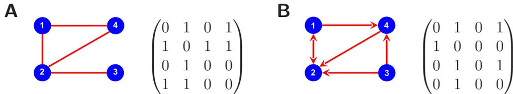
**Figure 1.5.** The adjacency matrix. An undirected network is shown on (A) and a directed network on (B). Notice that the diagonals of the matrices only contain zeros and that the undirected network has associated a symmetric matrix.
