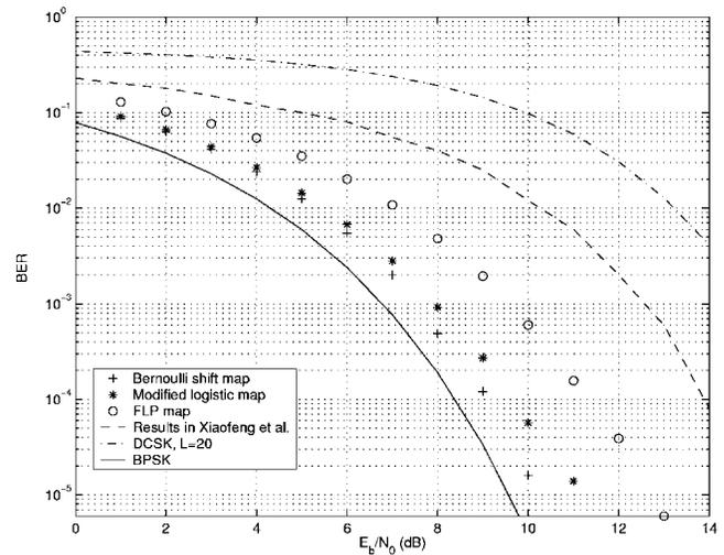
FIG. 13. BER performance for the Bernoulli shift, the modified logistic and the FLP maps, in the case of *BCJR decoding*, with  $P=32$  states and  $L=10$  symbols. The performance of BPSK (Ref. 21), DCSK (Ref. 2)  $L=20$  and other recent results (Ref. 25) are shown for comparison.
