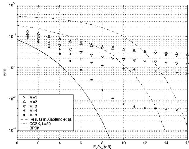
FIG. 5. BER against  $E_b/N_0$  for the modified logistic map in the case of heuristic decoding, with  $D=20$  bits and  $M=1, 2, 3, 4, 8$  symbols. The performance of BPSK (Ref. 21), DCSK (Ref. 2) with  $L=20$  and other recent results (Ref. 25) are shown for comparison.
