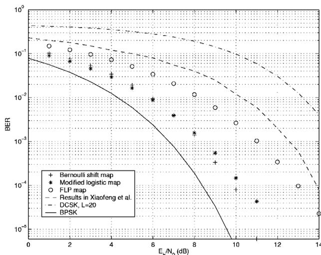
FIG. 12. BER against  $E_b/N_0$  for the Bernoulli shift, the modified logistic and the FLP maps, in the case of *Viterbi decoding*, with  $P=32$  states and  $L=10$  symbols. The performance of BPSK (Ref. 21), DCSK (Ref. 2) with  $L=20$  and other recent results (Ref. 25) are shown for comparison.
