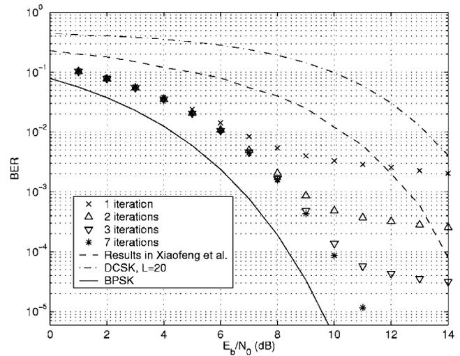
FIG. 9. BER against  $E_b/N_0$  for the Bernoulli shift map in the case of recursive heuristic decoding, with  $D=20$  bits,  $M=4$  symbols and 1, 2, 3, 7 iterations. The performance of BPSK (Ref. 21), DCSK (Ref. 2) with  $L=20$  and other recent results (Ref. 25) are shown for comparison.
