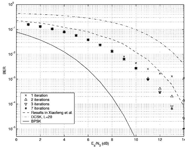
FIG. 11. BER against  $E_b/N_0$  for the FLP map in the case of *recursive heuristic decoding*, with  $D=20$  bits,  $M=4$  symbols and 1, 2, 3, 7 iterations. The performance of BPSK (Ref. 21), DCSK (Ref. 2) with  $L=20$  and other recent results (Ref. 25) are shown for comparison.
