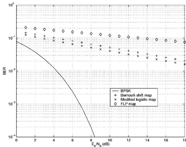
FIG. 3. BER against  $E_b/N_0$  in the case of direct decoding of the  $y_n$  sequence for each of the possible encoders based upon the Bernoulli, the modified logistic and the FLP maps. The BER of BPSK (Ref. 21) is shown for comparison.
