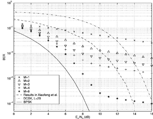
FIG. 4. BER against  $E_b/N_0$  for the Bernoulli shift map in the case of heuristic decoding, with  $D=20$  bits and  $M=1, 2, 3, 4, 8$  symbols. The performance of BPSK (Ref. 21), DCSK (Ref. 2) with  $L=20$  and other recent results (Ref. 25) are shown for comparison.
