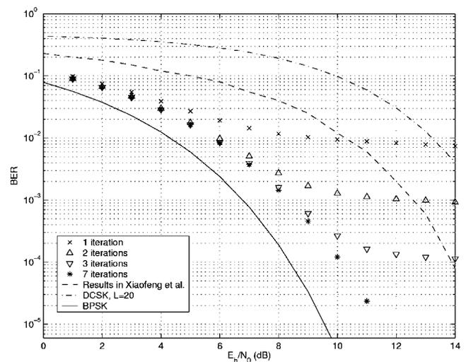
FIG. 10. BER against  $E_b/N_0$  for the modified logistic map in the case of recursive heuristic decoding, with  $D=20$  bits,  $M=4$  symbols and 1, 2, 3, 7 iterations. The performance of BPSK (Ref. 21), DCSK (Ref. 2) with  $L=20$  and other recent results (Ref. 25) are shown for comparison.
