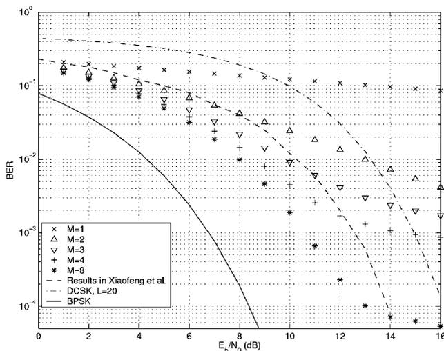
FIG. 6. BER against  $E_b/N_0$  for the FLP map in the case of heuristic decoding, with  $D=20$  bits and  $M=1, 2, 3, 4, 8$  symbols. The performance of BPSK (Ref. 21), DCSK (Ref. 2) with  $L=20$  and other recent results (Ref. 25) are shown for comparison.
