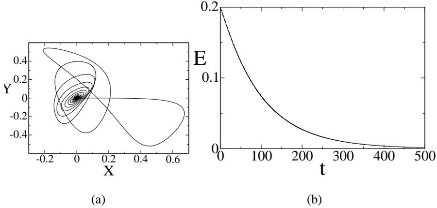
FIG. 4: (a) In the presence of dissipation ( $\alpha = 0.1$  and  $\beta = 0.1$ ), a particle permanently trapped in the scattering region. The corresponding trajectory approaches the fixed-point attractor in the phase space. (b) Exponential decay to zero of the particle energy when it approaches the attractor.
