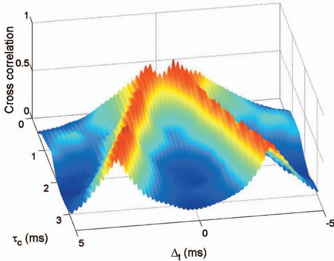
FIG. 2. (Color) Cross-correlation plot of Chua circuits A and B, as a function of the time shift  $\Delta t$  between both series and the time delay  $\tau_c$ . We can observe how the highest correlation ( $C_{\max} \sim 0.64$ ) always occurs at  $\Delta t = \pm \tau_c$ , which indicates that we have lag synchronization with exchanges in the leader-follower roles between both circuits.
