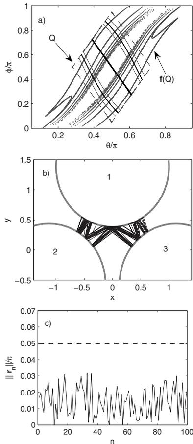
FIG. 5. Square  $Q$  (dashed), its image under  $\mathbf{f}$  (gray), and the sets  $S^0$  (thick black),  $S^1$  (black), and  $S^2$  (gray) for the three-disk scattering problem (a). A partially controlled trajectory when  $u_0=0.05\pi$  (b) and the control applied  $\|\mathbf{r}_n\|$  each bounce against the disk 1 (c), which clearly verifies  $\|\mathbf{r}_n\| < u_0$  (dashed line) as expected.
