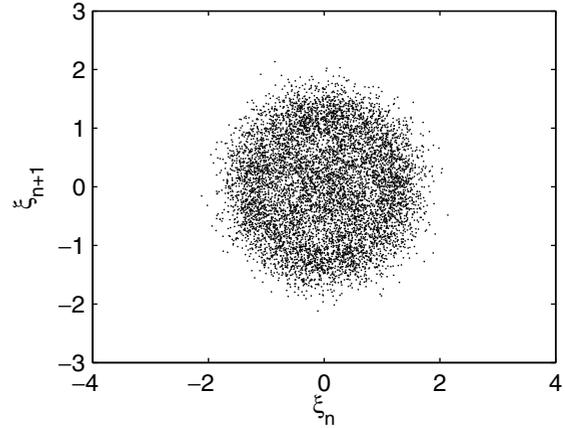
Fig. 1. Return map for a time series of the Lorenz map contaminated with Gaussian white noise with  $\sigma = 0.25$  (SNR  $\simeq 10$  dB). The structure of the underlying chaotic attractor has been totally blurred. However, the count of forbidden order patterns is sensibly higher than in the purely random case.
