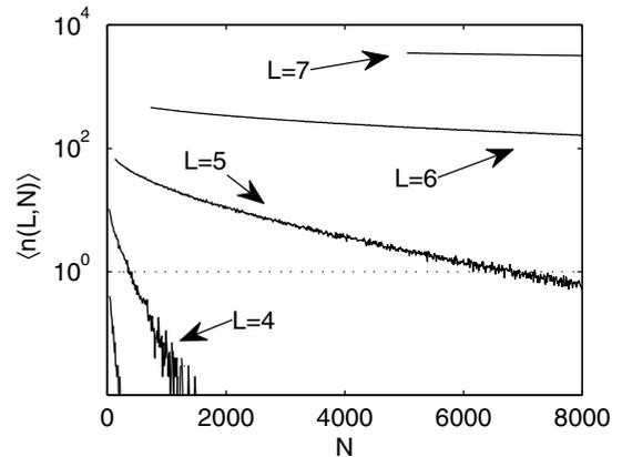
Fig. 7. Average number of forbidden patterns of length  $L$  found in a time series of length  $N$ ,  $\langle n(L, N) \rangle$ , (in logarithmic scale) for a noisy series of the time-delayed Hénon map with  $\sigma = 0.5$  (SNR  $\simeq 1.3$  dB).
