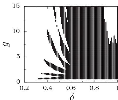
**Fig. 7.** Undamped signal propagation regions represented by black colour in the  $(\delta, g)$  parameter space for the coupled Bellows maps. The values of the other parameters in Eq. (6) are  $b = 2$ ,  $r = 2$ ,  $f = 0.1$ ,  $\omega = 0.1$ ,  $\Omega = 1$  and  $m = 100$ .
