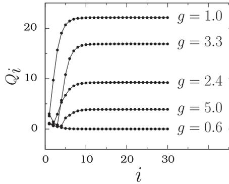
**Fig. 8.** Sigmoid function type variation of  $Q_i$  with  $i$  for  $\delta = 0.55$  and a few fixed values of  $g$  in the coupled Bellows maps. For  $g = 0.6$  a damped signal propagation takes place. For other values of  $g$ , an undamped signal propagation is realized.
