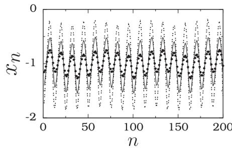
**Fig. 5.** Plot of  $x_n$  versus  $n$  for the Rulkov map at three values of  $g$  and with  $f = 0.005$ ,  $\omega = 0.1$  and  $\Omega = 0.5$ . The values of  $g$  for the dotted curve (inner most curve), continuous line curve (middle curve) and the dashed curve (outer most curve) are 0.1, 0.23 and 0.4 respectively. The resonance occurs at  $g = 0.23$ .
