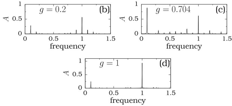
**Fig. 1.** Amplitude of the various frequency components of the solution of the Bellows map driven by the biharmonic signal  $F(n) = f\cos \omega n + g\cos \Omega n$ ,  $\Omega \gg \omega$ , for three values of  $g$ . The rest of the parameters fixed at  $b = 2$ ,  $r = 2$ ,  $f = 0.1$ ,  $\omega = 0.1$  and  $\Omega = 1$ . The spectrum has dominant peaks only at the frequencies  $\omega$  and  $\Omega$ .
