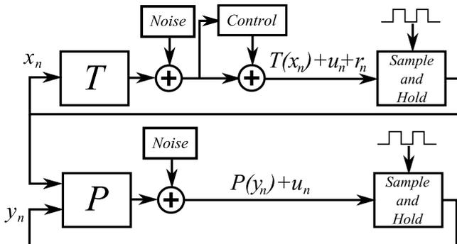
Fig. 11. Block diagram of the 2D system. The diagram is similar to the one-dimensional system but with an additional block that implements the function  $P$  and samples the variable  $y_n$ .
