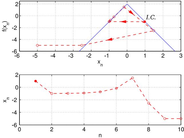
Fig. 6. Time series without control. The trajectory of the time series tends rapidly after a few iterations to  $-5$  V which is the saturation voltage of the circuit. The initial condition is displayed as I.C. in the figure and is marked with a red dot. The order of the iterations are marked with an arrow.
