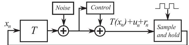
Fig. 3. Block diagram of the circuit. This schematic view of the algorithm shows the relation and the order between each block. The electronic circuit is constructed according to this representation.
