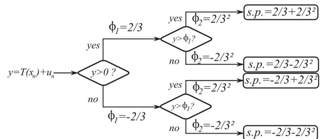
Fig. 4. State flow diagram of the implementation of the control method with the circuit, where “s.p.” means safe point.
