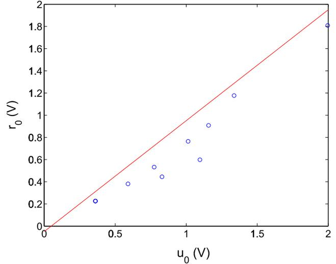
Fig. 8. The figure shows measurements of the maximum noise  $u_0$  against the maximum control  $r_0$ . Each point represents the maximum of a time series with different noise standard deviation. The solid line represents the unit line  $u_0 = r_0$ . All the points below this line satisfy  $r_0 < u_0$ .
