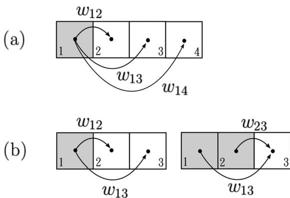
FIG. 8. (a) First, second, and third order transitions in a suppressing line. Since longer transitions contribute less or equal than shorter ones, we have  $w_{12} \geq w_{13} \geq w_{14}$ . This explains the monotonic decreasing character of  $w$ . (b) Two suppressing lines having the same total suppressibility but different number of black pixels or chaoticity. Note that  $w_{12} = w_{23} = 1$ .
