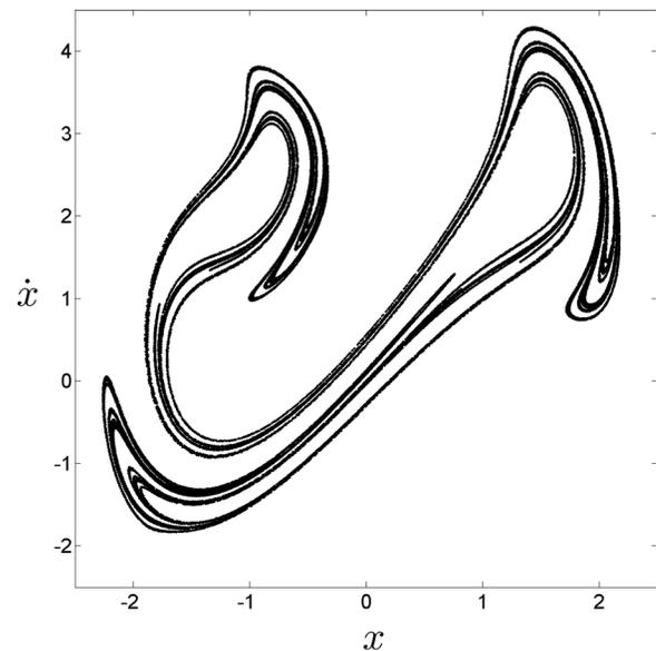
FIG. 1. Chaotic attractor for the Duffing oscillator  $\ddot{x} + 0.1\dot{x} - x + x^3 = 6.3 \sin t$ , with initial conditions  $(x, \dot{x}) = (1, 0)$ .
