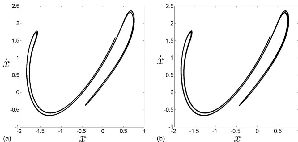
FIG. 4. (a) Chaotic attractor for the Duffing oscillator  $\ddot{x} + 0.34\dot{x} - x + x^3 = 6.8 \sin t$ . (b) Same chaotic attractor, though letting the driving amplitude fluctuate randomly in the interval  $[6.76, 6.84]$ , what corresponds to an uncertainty  $\Delta F = 0.04$ . This attractor looks a bit thicker, but preserves the shape.
