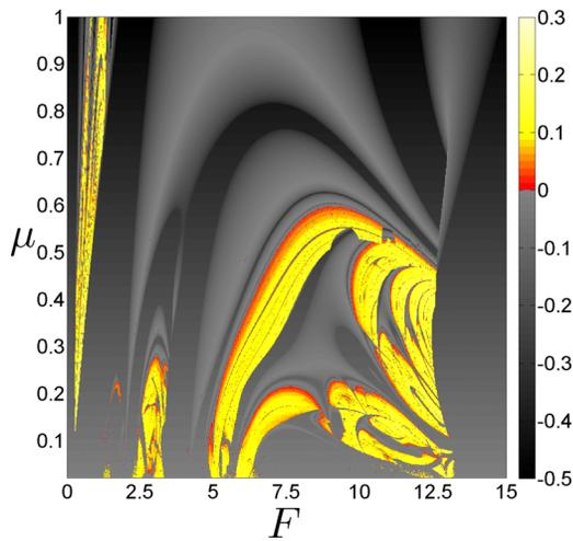
FIG. 2. Chaotic parameter set for the Duffing oscillator  $\ddot{x} + \mu\dot{x} - x + x^3 = F\sin t$  in the  $(F, \mu)$  parameter space. The color bar shows the value of the largest Lyapunov exponent, computed for a grid of  $720 \times 720$  points, and using as initial condition  $(x, \dot{x}) = (1, 0)$ . Both periodic (gray colored) and chaotic (non-gray colored) motions are displayed.
