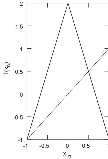
**Fig. 1.** The tent map with escapes  $x_{n+1} = T(x_n)$  where  $T(x) = \lambda(1 - |x|) - 1$  and  $\lambda = 3$ . There is a chaotic saddle in the  $[-1, 1]$  interval, from which nearly all trajectories (except a zero-measure set) escape under iterations.
