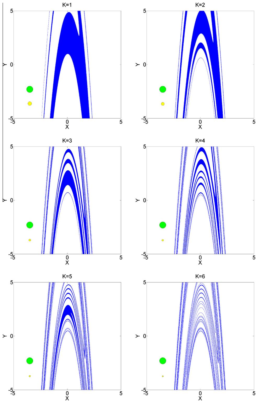
**Fig. 7.** We show here in blue the safe sets for the Hénon map for  $a = 2.16$  for different values of  $k$ . The green ball is the maximum admissible disturbance and the yellow ball the maximum admissible control, which clearly decreases with  $k$ . For every  $k$  we consider a constant disturbance with a maximum value equal to 0.3. (For interpretation of the references to colour in this figure caption, the reader is referred to the web version of this article.)
