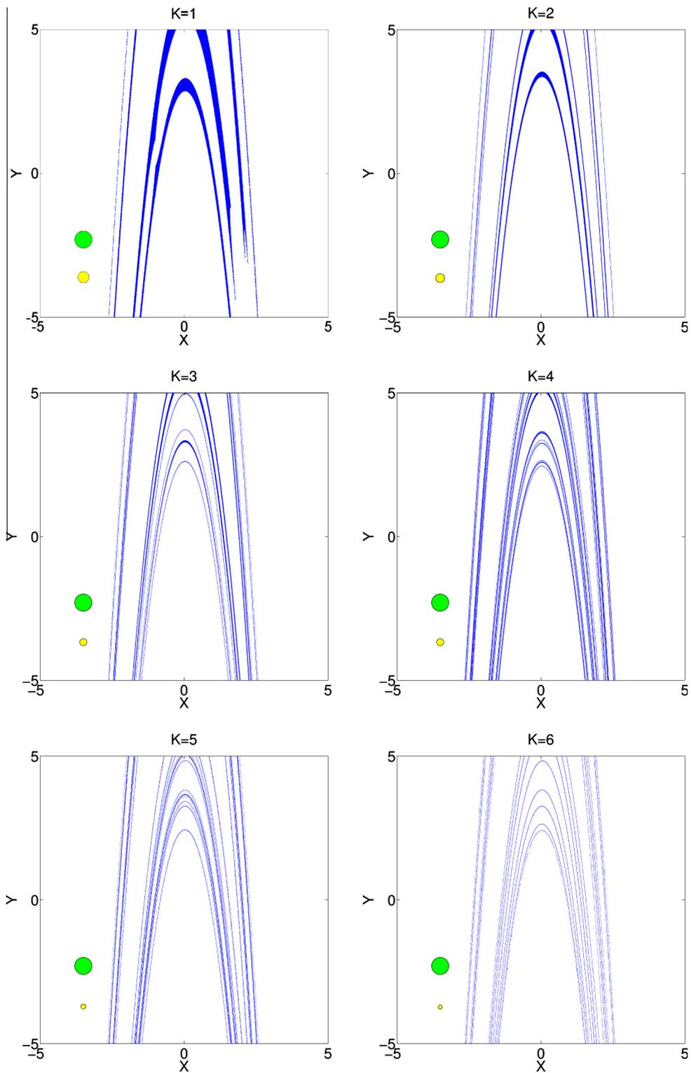
**Fig. 8.** We show here in blue the safe sets for the Hénon map for  $a = 3$  for different values of  $k$ . The green ball is the maximum admissible disturbance and the yellow ball the maximum admissible control, which clearly decreases with  $k$ . For every  $k$  we consider a constant disturbance with a maximum value equal to 0.3. (For interpretation of the references to colour in this figure caption, the reader is referred to the web version of this article.)
