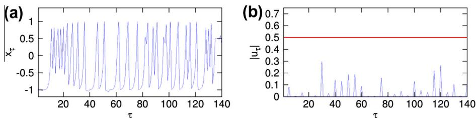
**Fig. 6.** A controlled trajectory of the tent map with a disturbance  $\xi_0 = 0.01$  when applying the control every  $k = 5$  iterations (the minimum control frequency) (a) and applied control (b). Note that the applied control is always smaller than the maximum allowed control in this example,  $u_{max} = 1$ .
