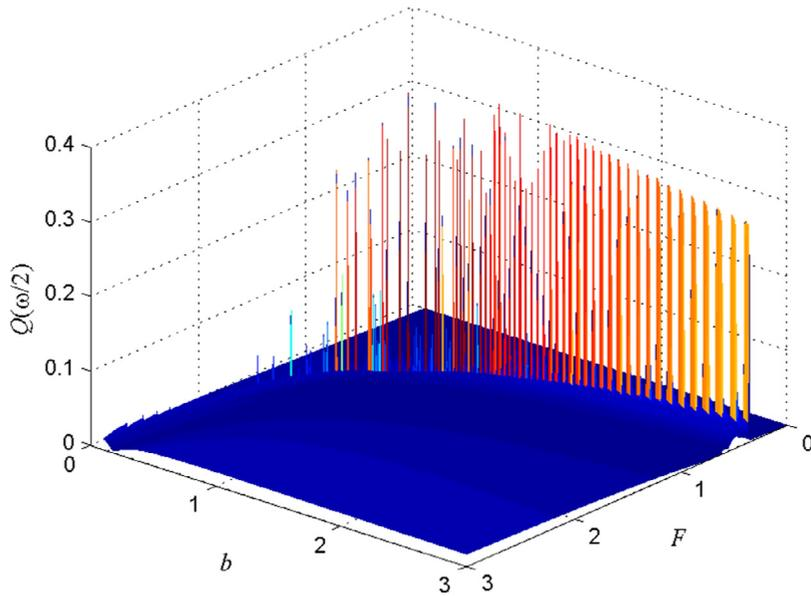
**Fig. 11.** The three-dimensional surface of the response amplitude  $Q(\omega/2)$  versus the nonlinear term coefficient  $b$  and the high-frequency excitation amplitude  $F$ , which indicates that the VSubR occurs at the subharmonic frequency  $\omega/2$ . The simulation parameters are  $a = 1$ ,  $f = 0.1$ ,  $\omega = 0.12$  and  $\Omega = 1$ .
