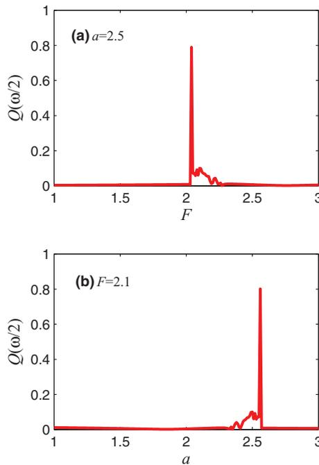
**Fig. 10.** The VSubR at the subharmonic frequency  $\omega/2$  induced by the high-frequency excitation amplitude  $F$  in (a) and induced by the linear coefficient term  $a$  in (b). The simulation parameters are  $b = 1$ ,  $f = 0.1$ ,  $\omega = 0.12$ ,  $\Omega = 1$ .
