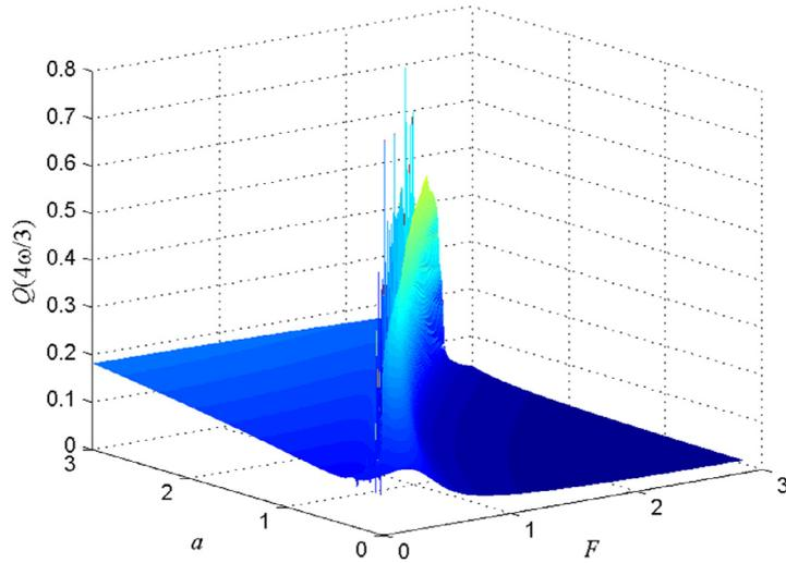
**Fig. 13.** The three-dimensional surface of the response amplitude  $Q(4\omega/3)$  versus the linear term coefficient  $a$  and the high-frequency excitation amplitude  $F$ , which indicates that the VSupR occurs at the superharmonic frequency  $4\omega/3$ . The simulation parameters are  $b = 1$ ,  $f = 0.1$ ,  $\omega = 0.12$  and  $\Omega = 1$ .
