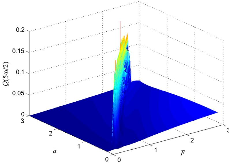
**Fig. 14.** The three-dimensional surface of the response amplitude  $Q(5\omega/2)$  versus the linear term coefficient  $a$  and the high-frequency excitation amplitude  $F$ , which indicates that the VSupR occurs at the superharmonic frequency  $5\omega/2$ . The simulation parameters are  $b = 1$ ,  $f = 0.1$ ,  $\omega = 0.12$  and  $\Omega = 1$ .
