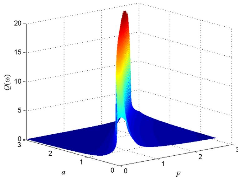
**Fig. 3.** The three-dimensional surface of the response amplitude  $Q(\omega)$  versus the linear term coefficient  $a$  and the high-frequency excitation amplitude  $F$ , which indicates that the traditional VR occurs at the primary frequency  $\omega$ . The simulation parameters are  $b = 1$ ,  $f = 0.1$ ,  $\omega = 0.12$  and  $\Omega = 1$ .
