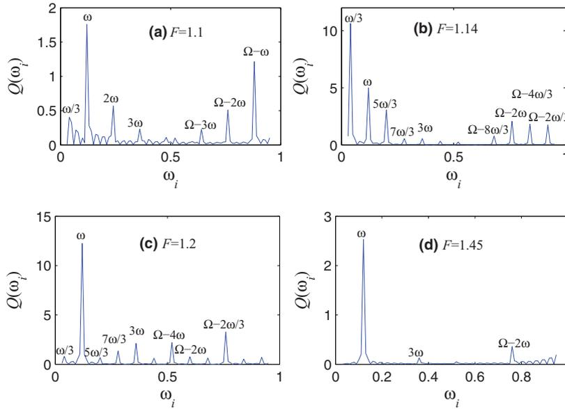
**Fig. 2.** The response amplitude  $Q(\omega_i)$  versus the frequency  $\omega_i$  for different values of  $F$ . The frequency  $\omega_i$  is the frequency existing in the low-frequency band in the response. The simulation parameters are  $a = 1.5$ ,  $b = 1$ ,  $f = 0.1$ ,  $\omega = 0.12$  and  $\Omega = 1$ .
