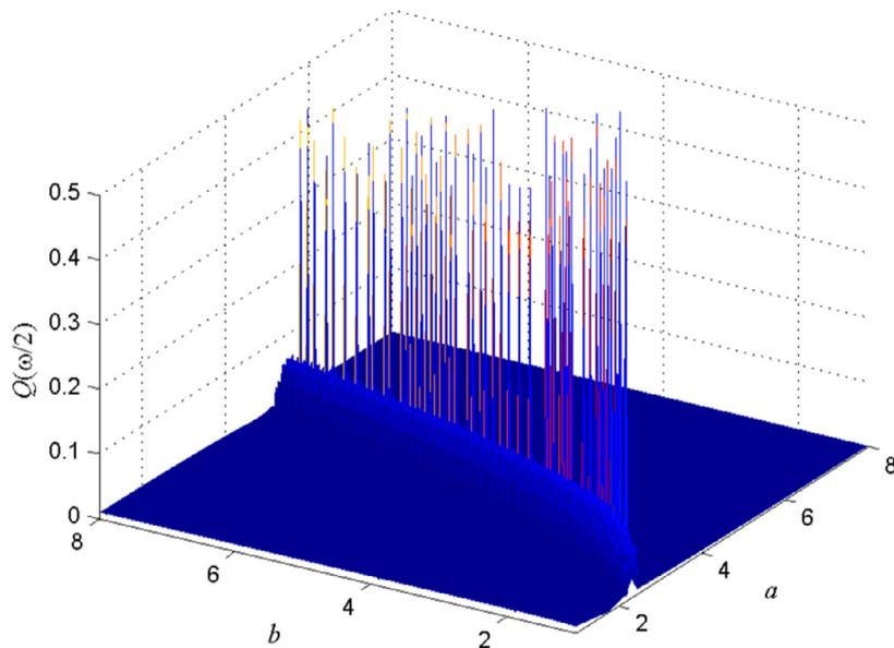
**Fig. 12.** The three-dimensional surface of the response amplitude  $Q(\omega/2)$  versus the linear term coefficient  $a$  and the nonlinear term coefficient  $b$ , which indicates that the VSubR occurs at the subharmonic frequency  $\omega/2$ . The simulation parameters are  $f = 0.1$ ,  $F = 2$ ,  $\omega = 0.12$  and  $\Omega = 1$ .
