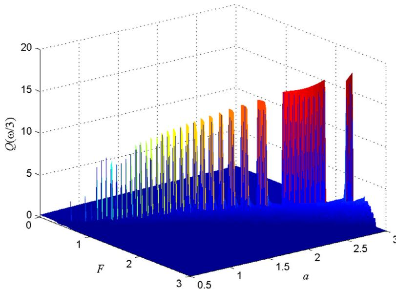
**Fig. 4.** The three-dimensional surface of the response amplitude  $Q(\omega/3)$  versus the linear term coefficient  $a$  and the high-frequency excitation amplitude  $F$ , which indicates that the VSubR occurs at the subharmonic frequency  $\omega/3$ . The simulation parameters are  $b = 1$ ,  $f = 0.1$ ,  $\omega = 0.12$  and  $\Omega = 1$ .
