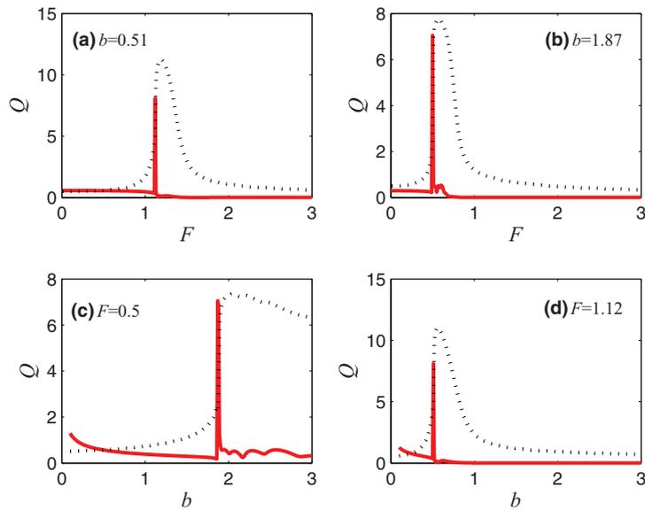
**Fig. 7.** Comparing VR and VSubR induced by the high-frequency excitation amplitude  $F$  in (a) and (b) and induced by the nonlinear term coefficient  $b$  in (c) and (d). The dotted line is  $Q(\omega)$  and the continuous line is  $Q(\omega/3)$  in each subplot. The simulation parameters are  $a = 1$ ,  $f = 0.1$ ,  $\omega = 0.12$ ,  $\Omega = 1$ .
