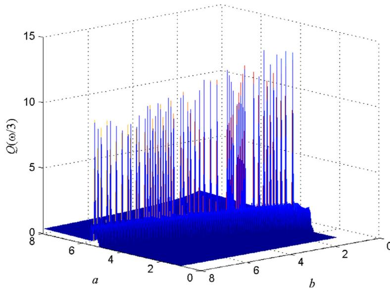
**Fig. 8.** The three-dimensional surface of the response amplitude  $Q(\omega/3)$  versus the linear term coefficient  $a$  and the nonlinear term coefficient  $b$ , which indicates that the VSubR occurs at the subharmonic frequency  $\omega/3$ . The simulation parameters are  $f = 0.1$ ,  $F = 2$ ,  $\omega = 0.12$  and  $\Omega = 1$ .
