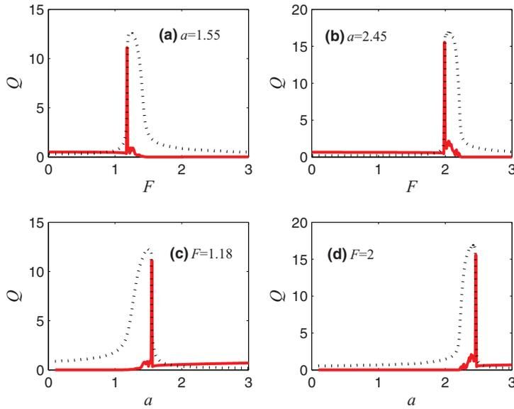
**Fig. 5.** Comparing VR and VSubR induced by the high-frequency excitation amplitude  $F$  in (a) and (b) and induced by the linear term coefficient  $a$  in (c) and (d). The dotted line is  $Q(\omega)$  and the continuous line is  $Q(\omega/3)$  in each subplot. The simulation parameters are  $b = 1$ ,  $f = 0.1$ ,  $\omega = 0.12$ ,  $\Omega = 1$ .
