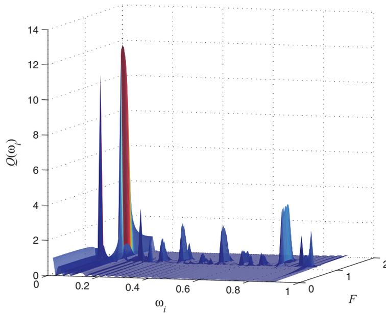
**Fig. 1.** The response amplitude  $Q(\omega_i)$  versus the high-frequency excitation amplitude on the three-dimensional plane. The frequency  $\omega_i$  is the frequency existing in the low-frequency band in the response. The simulation parameters are  $a = 1.5$ ,  $b = 1$ ,  $f = 0.1$ ,  $\omega = 0.12$  and  $\Omega = 1$ .
