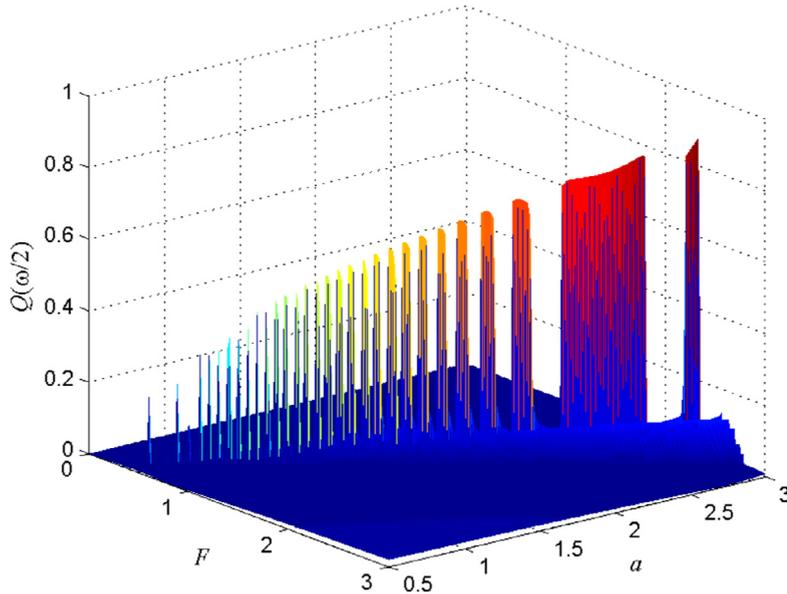
**Fig. 9.** The three-dimensional surface of the response amplitude  $Q(\omega/2)$  versus the linear term coefficient  $a$  and the high-frequency excitation amplitude  $F$ , which indicates that the VSubR occurs at the subharmonic frequency  $\omega/2$ . The simulation parameters are  $b = 1$ ,  $f = 0.1$ ,  $\omega = 0.12$  and  $\Omega = 1$ .
