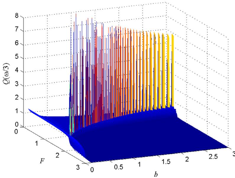
**Fig. 6.** The three-dimensional surface of the response amplitude  $Q(\omega/3)$  versus the nonlinear term coefficient  $b$  and the high-frequency excitation amplitude  $F$ , which indicates that the VSubR occurs at the subharmonic frequency  $\omega/3$ . The simulation parameters are  $a = 1$ ,  $f = 0.1$ ,  $\omega = 0.12$  and  $\Omega = 1$ .
