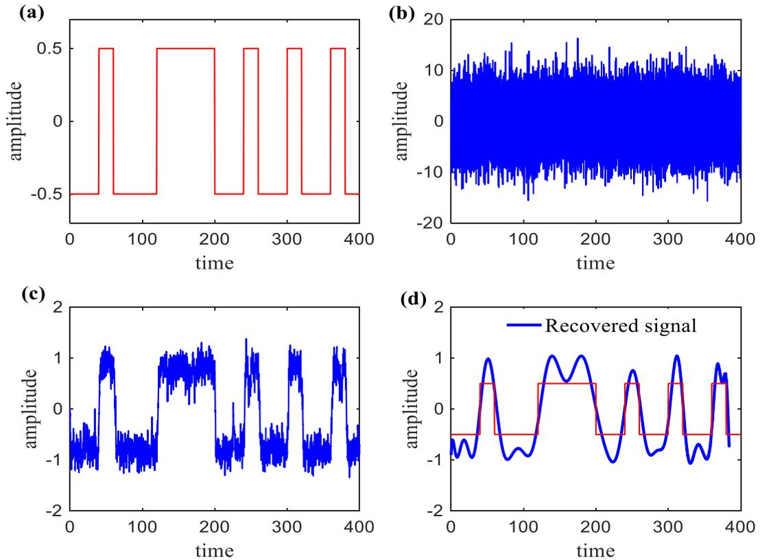
**Fig. 7.** The recovery of a binary signal. (a) The original binary signal, (b) binary signal totally buried by the strong Gaussian white noise, (c) the time-domain spectrum of the response of the nonlinear system, (d) recovered signal obtained by the polynomial fitting according to subfigure (c).
