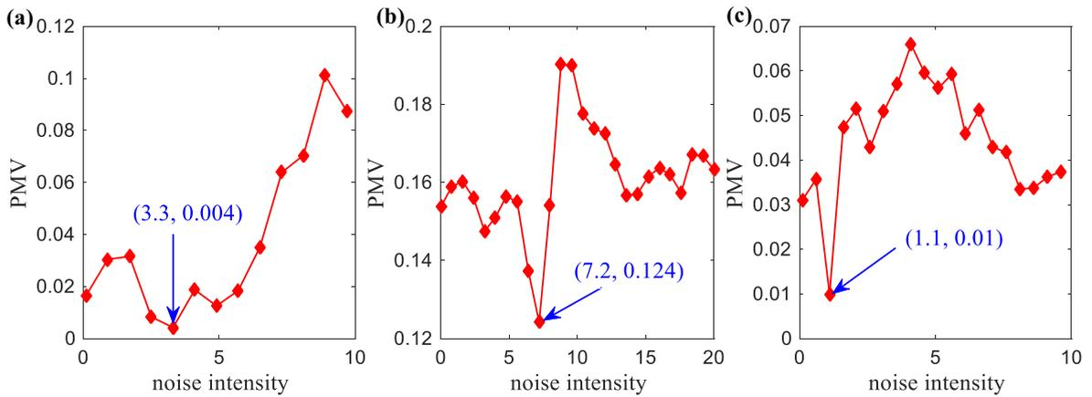
**Fig. 5.** The value of the PMV indicator depends on the noise intensity. (a) The signal to be restored is a harmonic signal. The minimum PMV is 0.004 when the noise intensity is  $D=3.3$ . (b) The signal to be restored is a binary signal. The minimum PMV is 0.124 when the noise intensity is  $D=7.2$ . (c) The signal to be restored is a chirp signal. The minimum PMV is 0.01 when the noise intensity is  $D=1.1$ .
