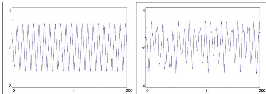
Fig. 4. Evolution of velocity over time for periodic and chaotic motions.
